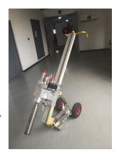
The HD-500AM is our powerful hydraulic core drill with a wide range of speeds and drilling capacity (Two speeds at the drilling gear and OK- hydraulic power packs offer three speeds. output six speeds), And excellent choice for heavy duty core drilling applications where high production rates are needed ,especially with large diameter core.
